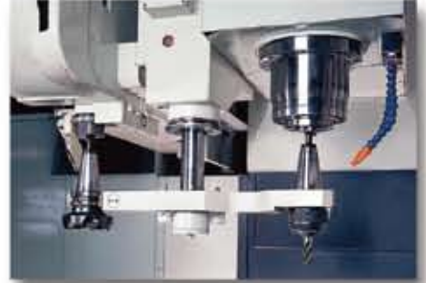
● ARM TYPE AUTOMATIC TOOL CHANGE 32 / 40 TOOLS 刀臂式自動換刀
