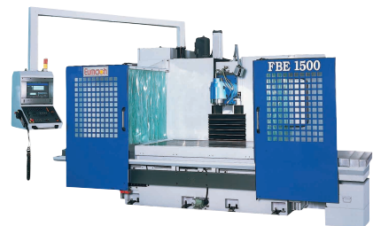
FBE SERIES BED TYPE MILLING MACHINES. X AXIS UP TO 4000MM. FBE系列萬能銑床
