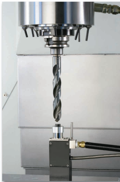
● RING TYPE COOLANT NOZZLES & TOOL LENGTH MEASUREMENT 主軸環狀冷卻噴水及刀長量測
