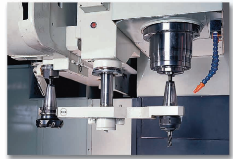
● ARM TYPE AUTOMATIC TOOL CHANGE 20 / 24 / 32 / 40 TOOLS 刀臂式自動換刀
