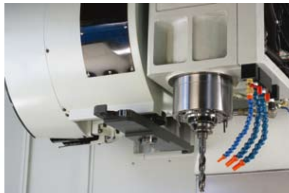
■ CAM type tool changer system 24/32 Tools刀臂式刀庫
