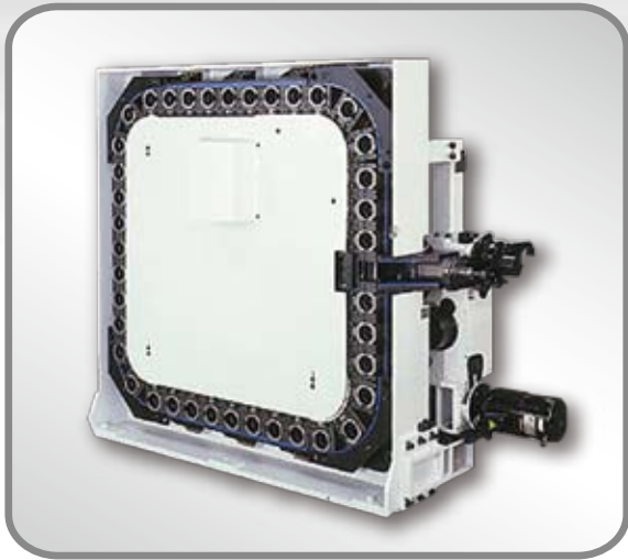
Standard 60 stations automatic tool changer with maximum 150mm diameter / 350mm length / 20 KG tool.
