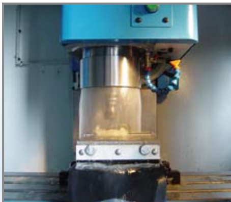
▲ Wet type graphite machining by water curtain & paper filtering
