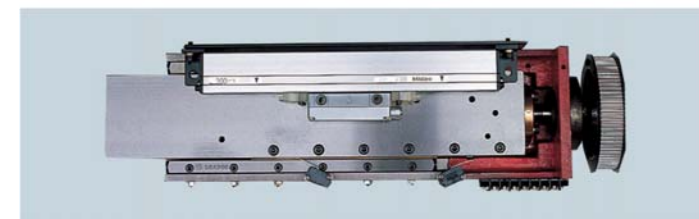
◆ The four sets of precise linear bearing in the servo spindle of Z-axis
