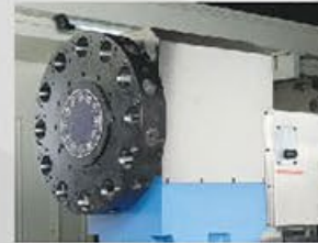
Baruffaldi TB Servo turret with VDI disc
