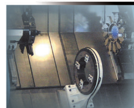
Option Application- LH: VDI Turret RH: 12-Angle Turret Steady Rest (Special Order Made)
