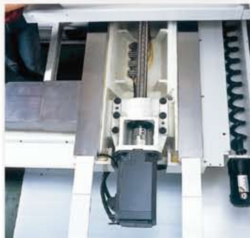
● DIRECTLY COUPLED BETWEEN BALLSCREW AND SERVO MOTOR (三軸直接傳動)
