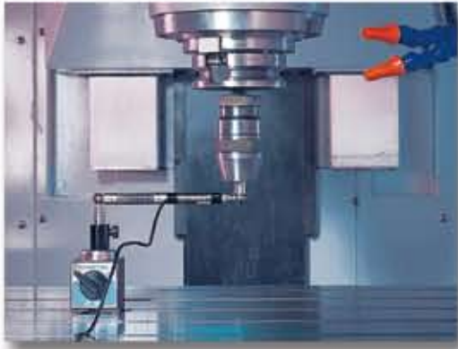
● BALL BAR TEST (循圓測試)
