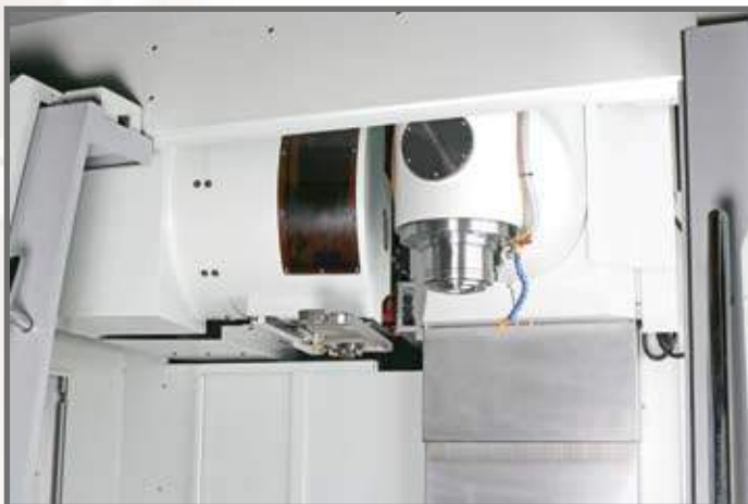
▶ MOVING 430MM FORWARD TO TOOLS CHANGING POSITION
